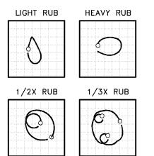
The severity of the rub will affect the shape of the orbit. A light rub will produce a "tear drop" shaped orbit, with the point of the teardrop coinciding with the impact spot. As the rub gets heavier the orbit will flattened and may appear as an excessive preload.
