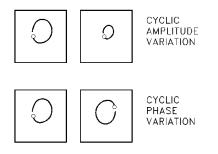
As the loose part rotates it influences the balance condition of the rotor, which appears as a cyclical, increase and decrease in the synchronous amplitude. This is observable using a spectrum analyzer, but the changes may be too rapid for the sampling rate of the instrument. An oscilloscope set up to observe a filtered orbit will sample continuously so that the changes can be seen. The phase shifting can, also, be observed using an oscilloscope.
