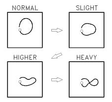
As the preload increases the orbit is further flattened. As excessive preload increases further the orbit begins to collapse to form a "banana" shape as the shaft tries to continue its normal rotation pattern and direction.
